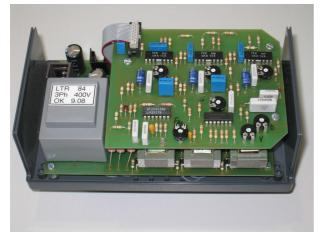
The 3 Phase LTR (PLR) Power Load Regulator consists of a Power Unit and a Control Unit. The Power Unit comprises the following components: 3 thyristors (3 modules), inductance choke coils, antiinterference capacitors and a generator protective contact breaker.
